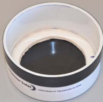
80mm refactor filter - foamcore ring inside held with silicone glue
