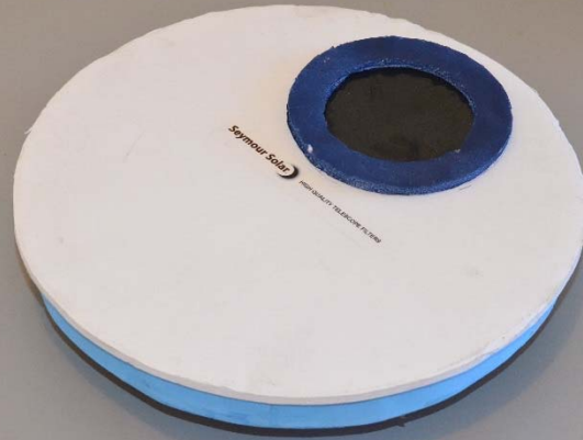
200mm SCT filter - foamcore and cardboard
