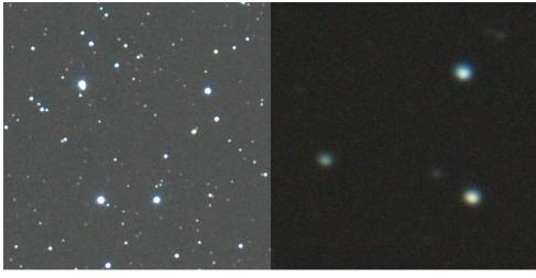
On the night of February 19th I got a chance to test the new auto-guider at Hallam Observatory. The photos at right show the central 400 x 400 pixels of two images from my Canon 5D MkII. The image on the left is through the AT111 and the right is the C-14. Exposures were 10 minutes and auto-guided on an 8th magnitude star.
