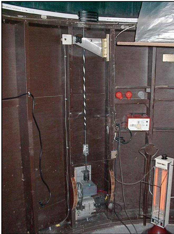
The dome rotation project is complete. As seen in this photo all moving parts are safely covered by Plexiglas. A wheel at the top of the mechanism runs on the dome track and the entire dome rotates by friction which can be adjusted by the black knob.
