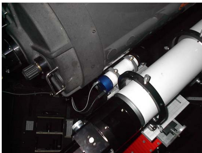
Autoguider (finderscope with blue camera) in its' new location
