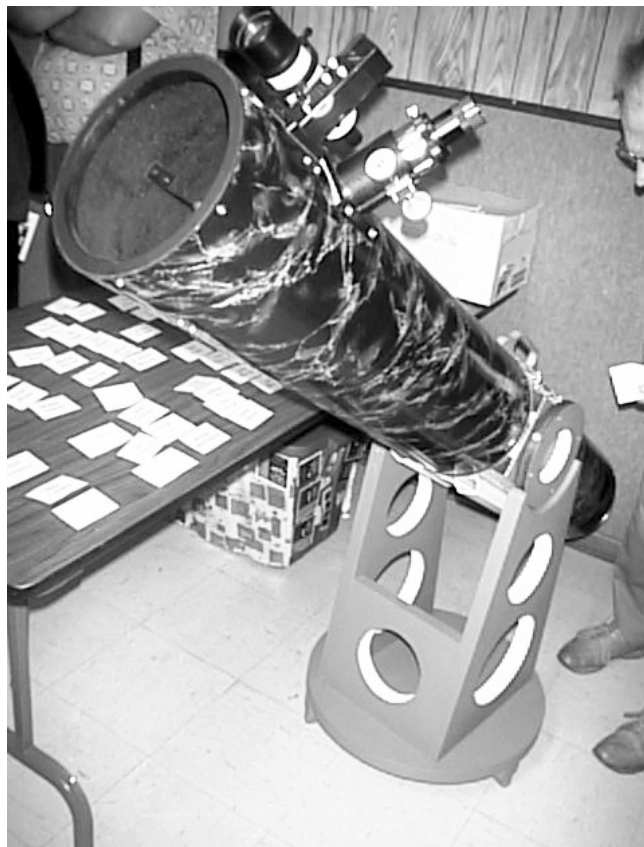
Dave Panton presented the club with his latest creation at the November General Meeting. Dave converted the old Gus Nyberg telescope into this very lightweight and portable 8" dobsonian style reflector. Members in attendance at the meeting got a chance to share in the "first light" views through the telescope by observing the penumbral lunar eclipse.
